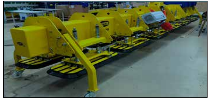
Figure 8: Blade Demolding Device
