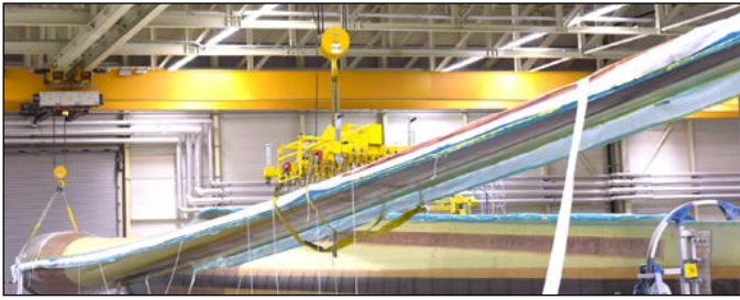
Figure 7: Transporting the Rotor Blade with Demolding Beam on the Tip Side
