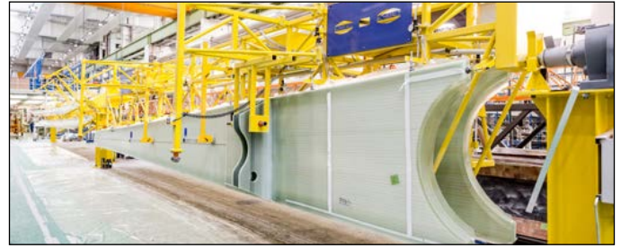
Figure 5: Aligning and Positioning the Webs
