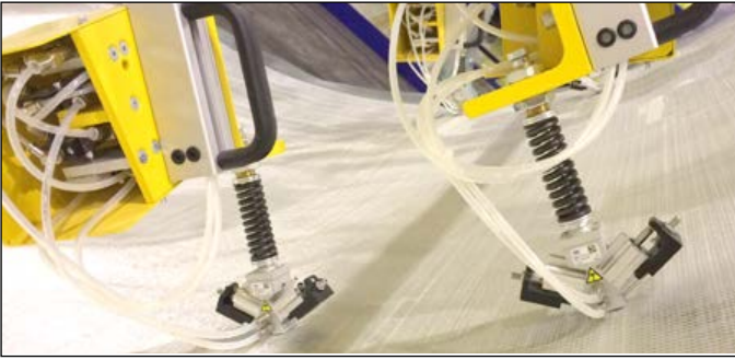
Figure 2: Handling of Composites by means of a Needle Gripper
