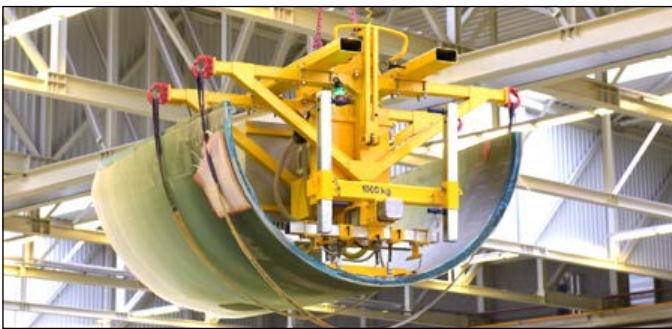
Figure 3: Transporting the Root Element for Installation
