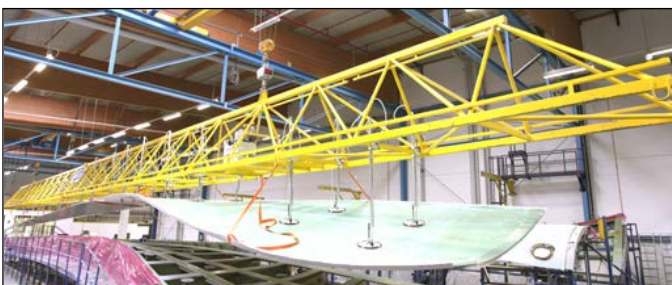
Figure 4: Handling the Rotor Blade Segment
